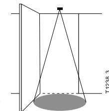
If the door is already in motion, its movement is not interrupted by the safety devices for the swing area.
